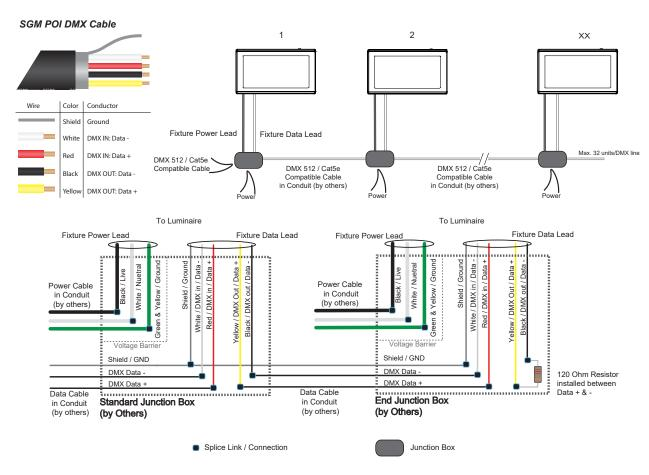
Figure 19: Connecting DMX and AC Power in P-6 POI
