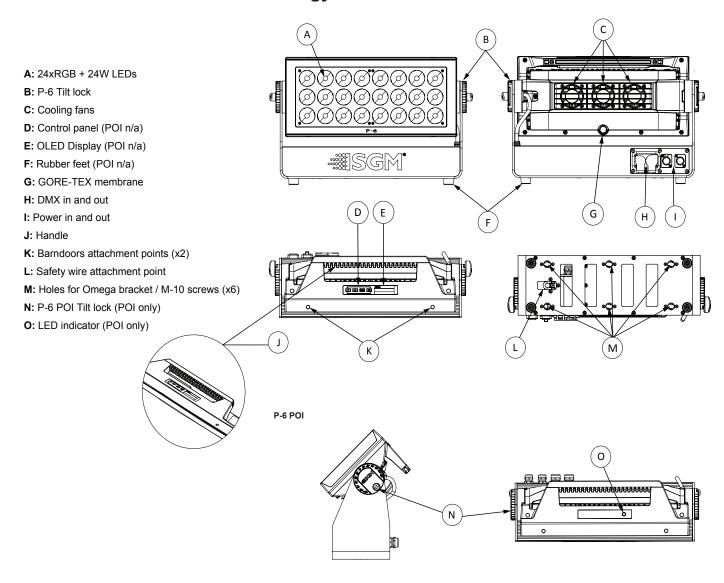
Figure 1: Parts identification and terminology
