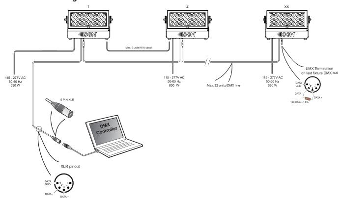
Figure 11: P-6 connection diagram (see "P-6 POI connection diagram" on page 18 for POI)
