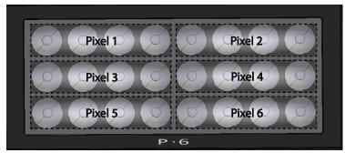
Figure 13: P-6 Pixel segments
