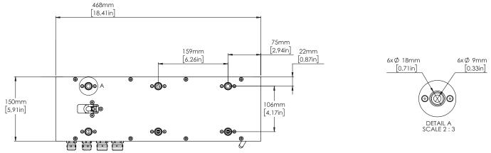
Figure 18: P-6 POI base with dimensions
