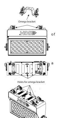
Figure 3: Base with omega bracket
